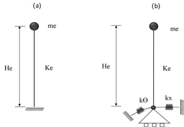
Fig. 5. (a) Idealized fixed base SDOF system, (b) Idealized system as uncoupled springs
