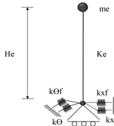
Fig. 7. Uncoupled springs after adding EPS foam to the system
