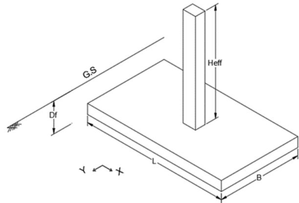
Fig. 4. Rectangular isolated footing dimensions
