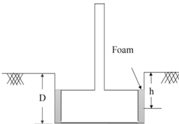
Fig. 2. SDOF system with EPS around the foundation
