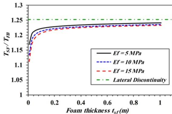
Fig. 8. Relation between  $T_{SF}$  and  $T_{FS}$  for a structure with an isolated footing on soft soil
