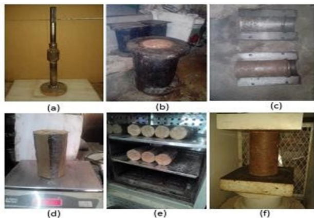
Fig. 2. Sequences involved in preparation and testing of UCS of cylinder specimens (a) Tamper used with vibratory hammer for compaction of cylindrical specimens, (b) Cylindrical mould (101.6 mm diameter and 203.2 mm height) used for compaction, (c) Removal of specimen from the mould after 24 hours, (d) Weighing of specimen after proper sealing, (e) Curing of specimens in the BOD incubator at a constant temperature (23±1.7°C) (f) Unconfined compression test of specimen (after 7 days) using a Compression testing machine
