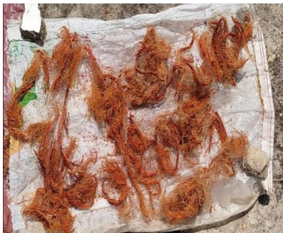
Fig. 1. Coconut coir fiber set up for sun drying
