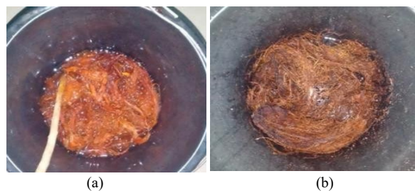
Fig. 2. Treatment of Coir Fiber with (a) NaOH and (b) Acetic acid solutions
