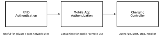
Fig. 2. RFID and mobile-app authentication concept for controlled charging access
