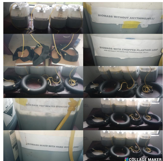
Fig. 1. Locally fabricated digester with gas collection tubes fixed
