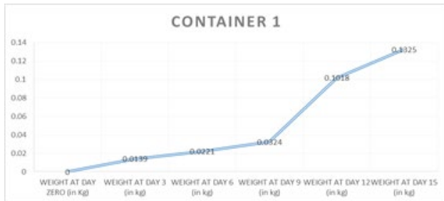
Fig. 2. Biogas production in container 1 for day 0-15
